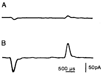
Fig. 15A and B. Capacitive current of a chromaffin cell. (A) After establishing a giga-seal on a chromaffin cell, a 20 mV pulse was applied to the pipette interior starting from a holding potential equal to the bath potential. The capacitance of the pipette and of the patch was almost completely compensated (see part I), resulting in very small capacitive artifacts. The pipette input resistance was 20 G \Omega . (B) After disruption of the patch the response to a 3 mV pulse at a holding potential of -54 mV was measured. The capacitive current was much larger than in A, as the cell membrane capacitance had to be charged (compare the amplitudes of the voltage steps). From the integral of the capacitive current a cell membrane capacitance of 5 pF is calculated. The cell had a diameter of 13 \mu m. Assuming a spherical shape, one obtains a unit capacitance of about 1 \mu F/cm ^2 . The DC current was smaller than 2 pA, indicating a cell membrane resistance of several G \Omega . The time constant of the capacitive current was less than 0.1 ms, which, together with the value of the cell capacitance, indicates a series resistance smaller than 20 M \Omega .
